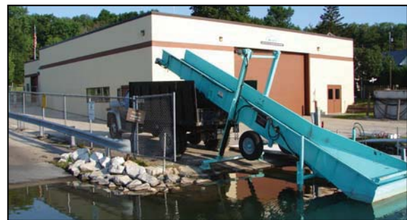
On Big Cedar Lake, weeds that are cut and gathered by a weed-cutting machine are transferred to a truck and disposed of off-site.
