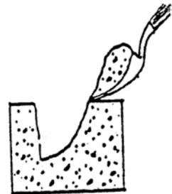
Push down on handle 4 inches to break slice; pull out on shovel with soil in one piece.
